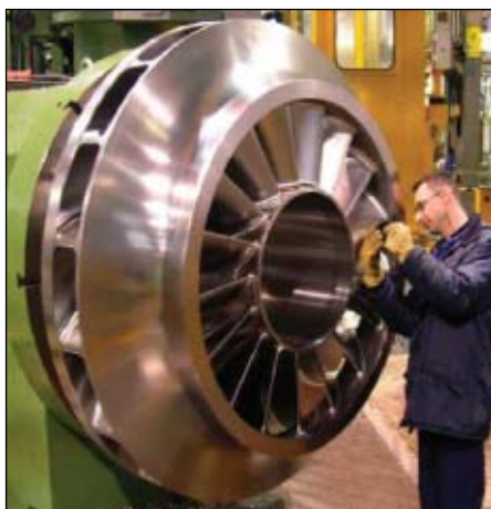
A worker inspects a single-piece 5-axis milled compressor impeller (Fig. 7; photograph from GE Oil & Gas, Florence).
