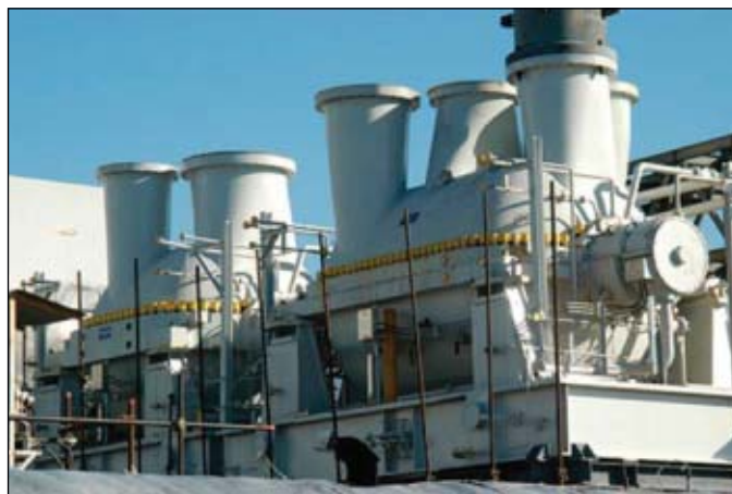
Compressor testing at Massa, Italy, shows GE’s propane compressors, the highest rated capacity of their type in the industry (Fig. 6; photograph from GE Oil & Gas, Florence).
